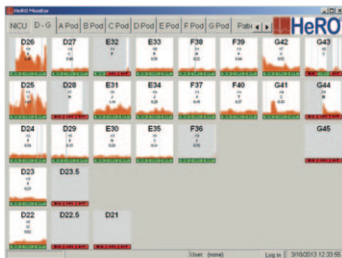
FIGURE 2 A 'pod view' from the HeRO monitor showing HeRO scores on multiple patients. In this view, five-day trends for five patients are shown by orange dotted lines and current HeRO scores are indicated in the right hand panels.
